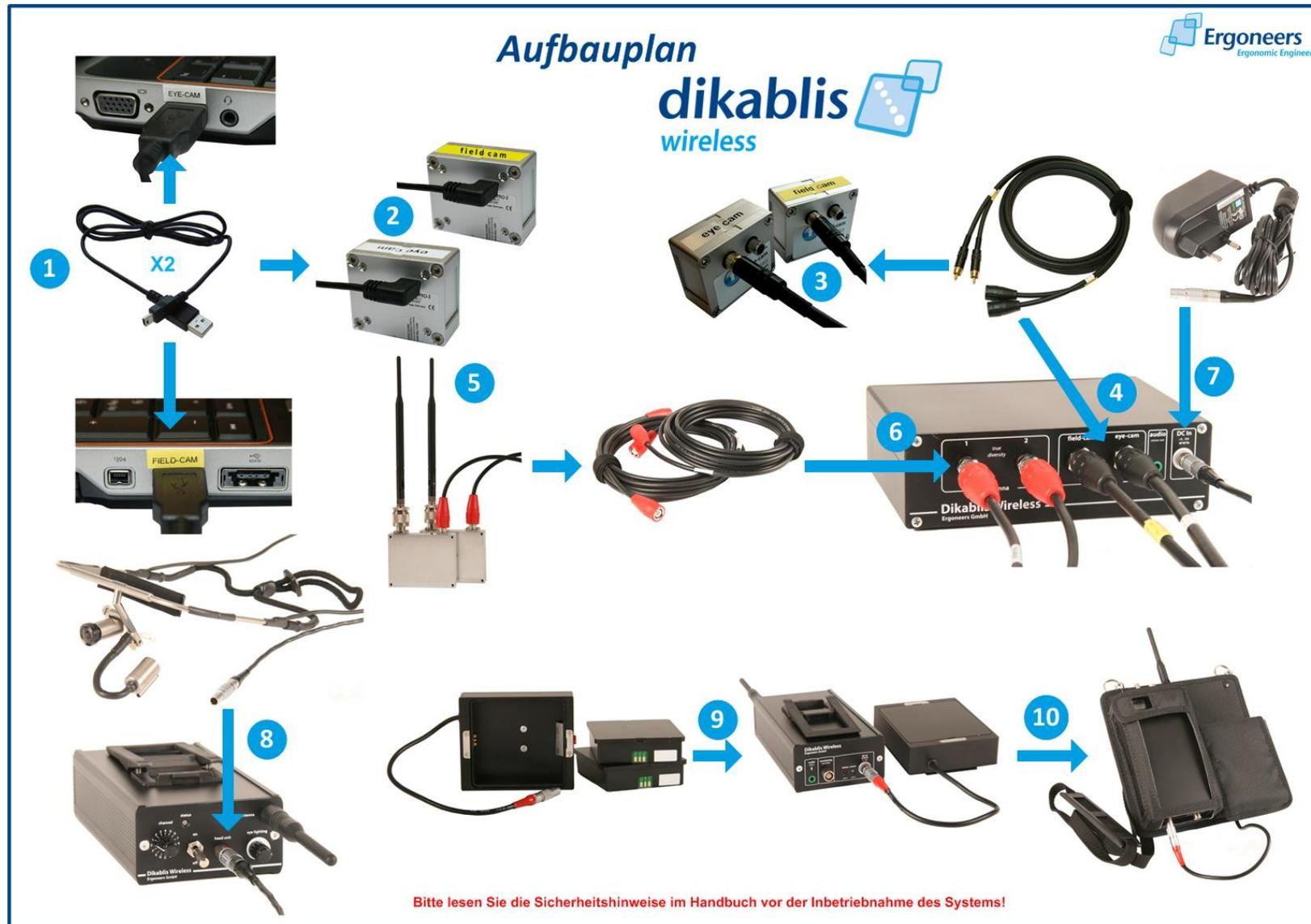
Figure 2-2: Dikablis Wireless set-up
