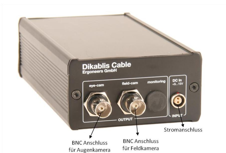
Figure 3-20: rear view of the Dikablis Cable electronic unit
