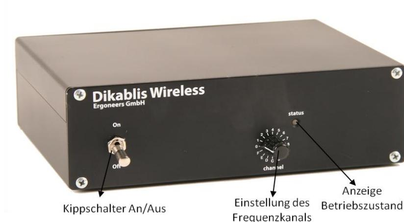
Figure 3-28: front view of the receiver
