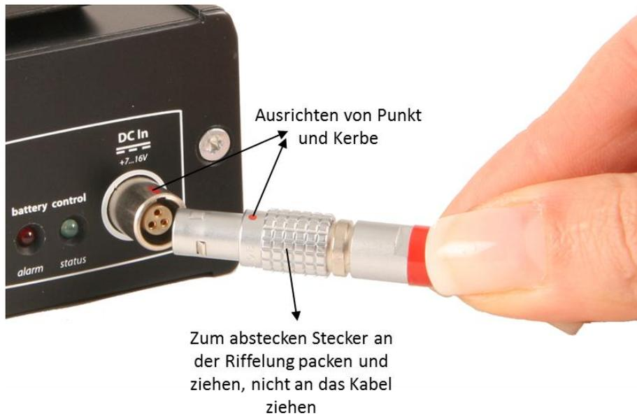
Figure 3-1: inserting the plug
