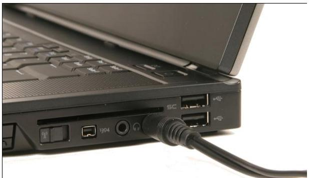
Figure 3-11: audio cable connection
