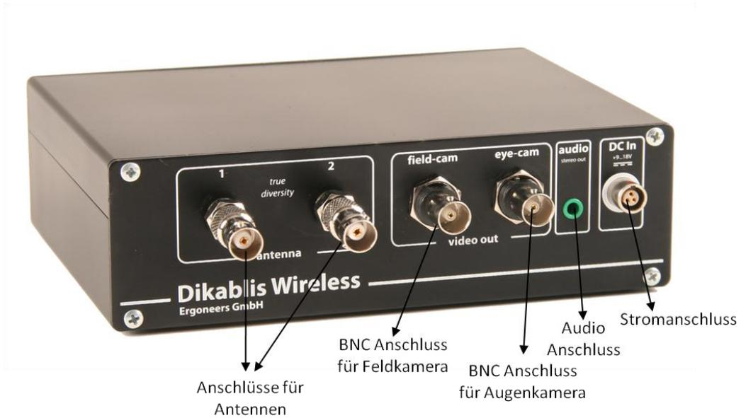
Figure 3-30: rear view of the receiver
