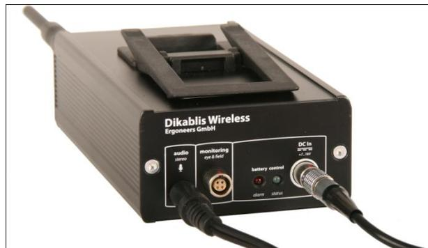
Figure 3-12: wireless audio connection (on the left)
