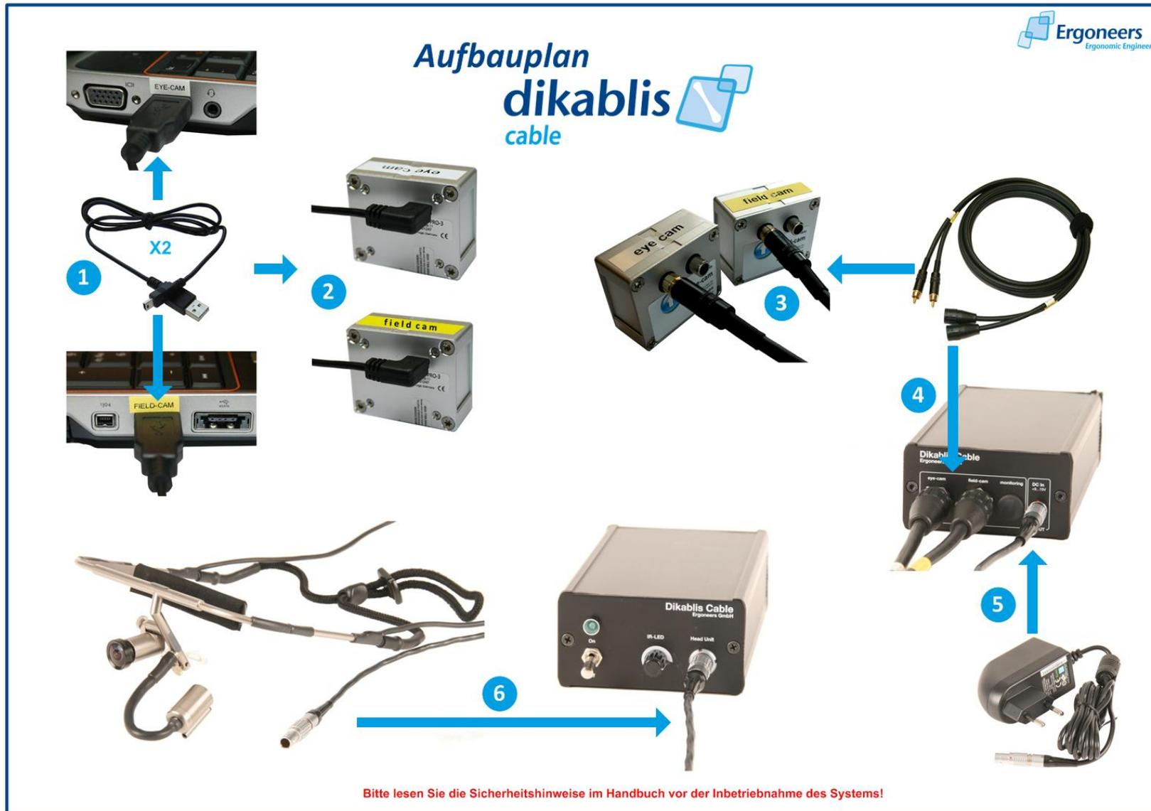
Figure 2-1: Dikablis Cable set-up
