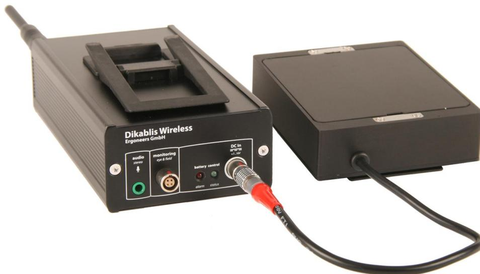
Figure 3-25: connection between the transmitter and the battery holder
