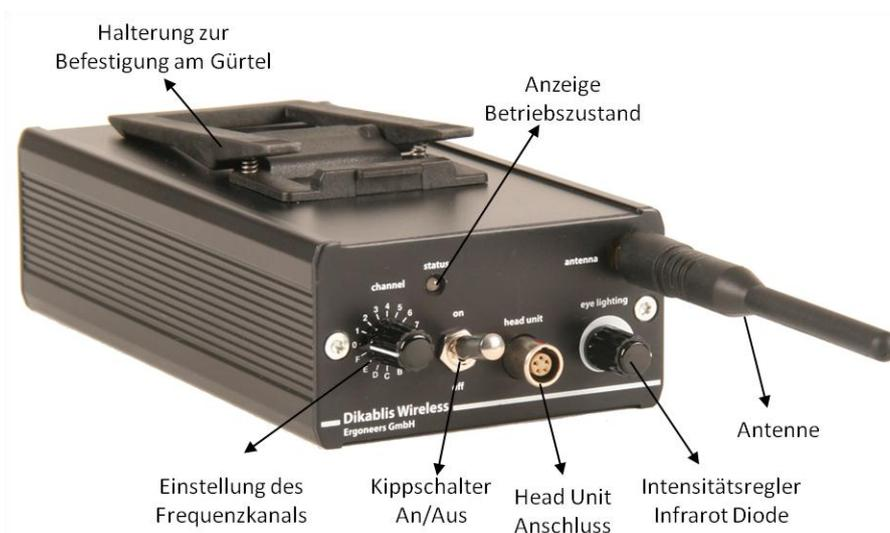
Figure 3-21: front of the transmitter
