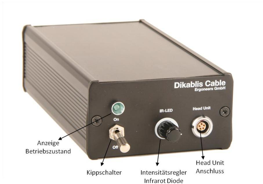
Figure 3-19: front view of the Dikablis Cable electronic unit
