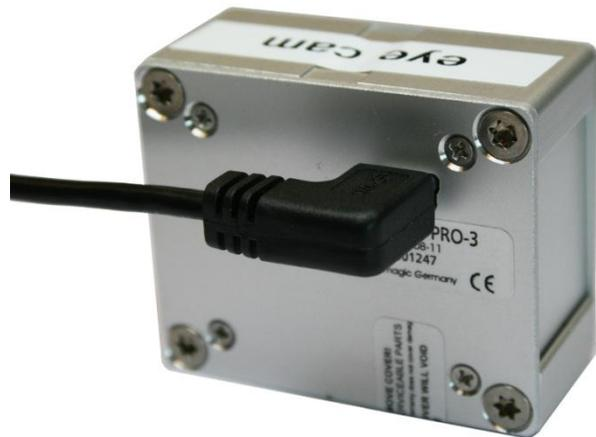
Figure 3-7: grabber box with connected mini USB cable
