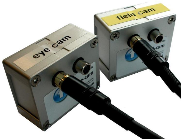
Figure 3-8: frame grabber box for the field and eye camera
