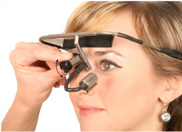
Figure 2-24: adjusting the field camera
