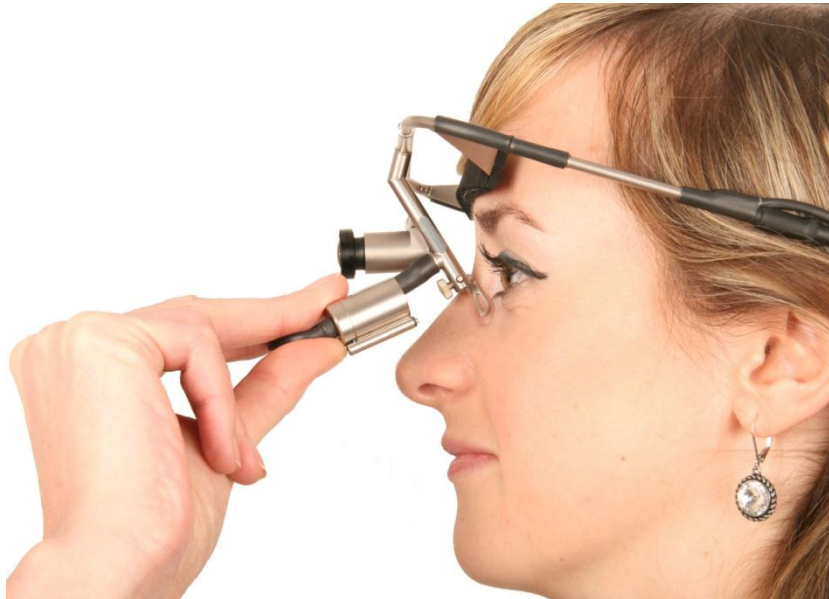
Figure 2-16: adjusting the eye camera
