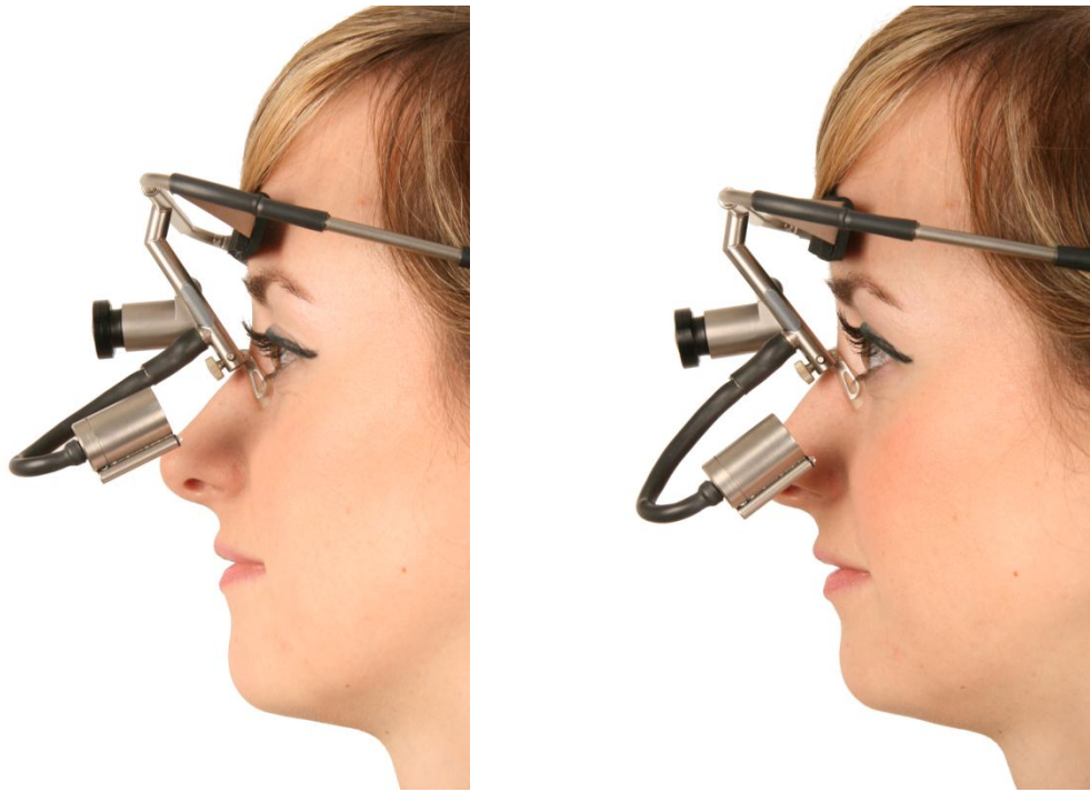
Figure 2-23: vertical position of the eye camera in relation to the eye
